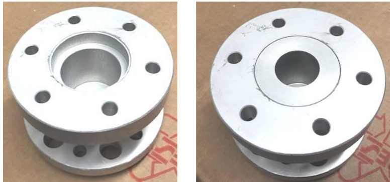
Engine side of spacer – without reducing washer, and with washer fitted.
